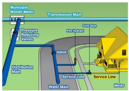
**Figure 1. Water Service Connection**
